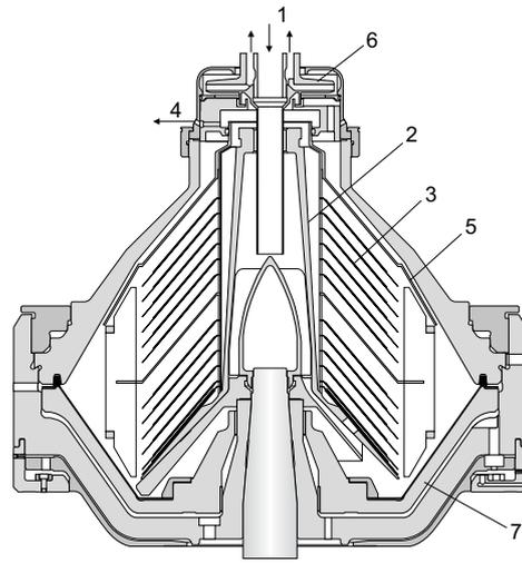
Typical bowl for a solids-ejecting centrifuge. The details illustrated do not necessarily correspond to the centrifuge described.
