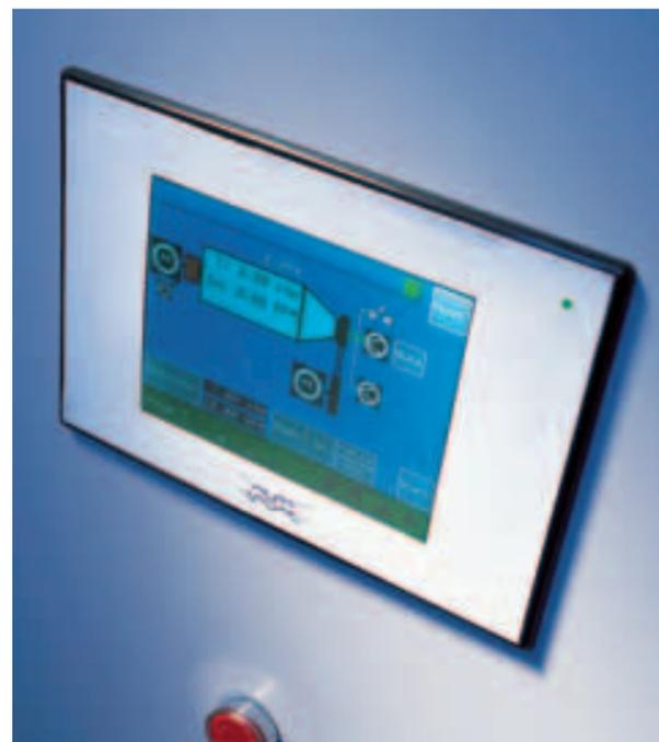
Screen for Decanter Core Controller (DCC)
