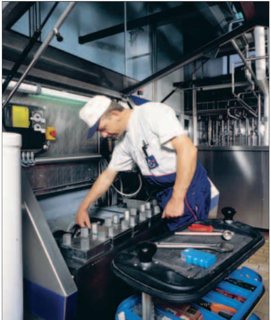
*Easy-to-open doors and removable covers make maintenance easy and accessible in Tetra Alex 400 homogenizers.*
