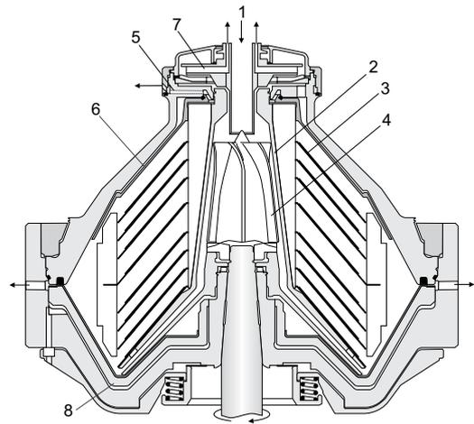
Typical bowl drawing for a solids-ejecting centrifuge (concentrator model). The details illustrated do not necessarily correspond to the centrifuge described.
