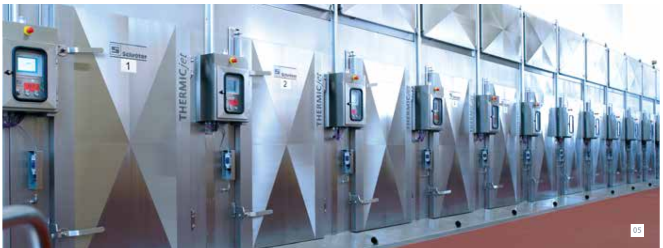
01-04 THERMICjets® for a variety of types of suspension rail conveyor systems 05 Hot-smoking system with four-trolley capacity
